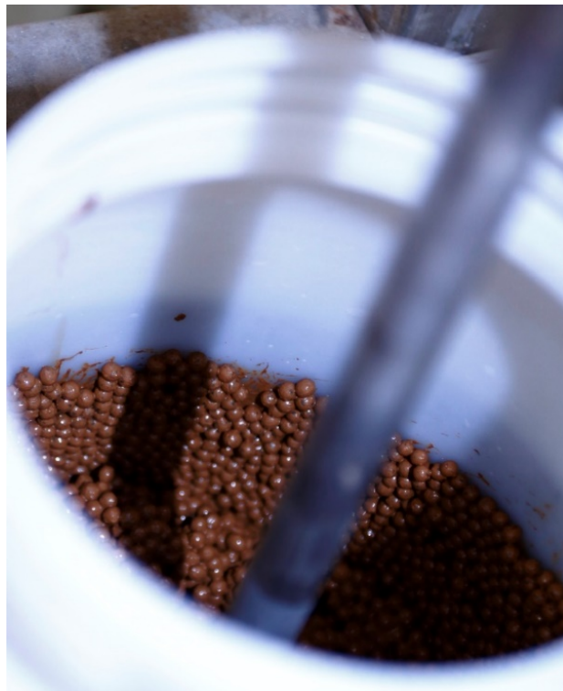
Figure 2: Laboratory scale low energy deagglomeration of -38 micron sample utilising glass beads as grinding media
