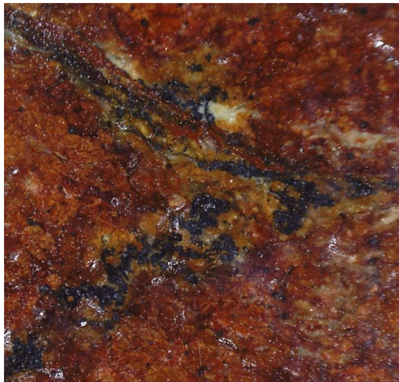
Figure 4: Photomicrograph of Polished Mt Thirsty drill core illustrating asbolane veins. Image is 4mm across.
